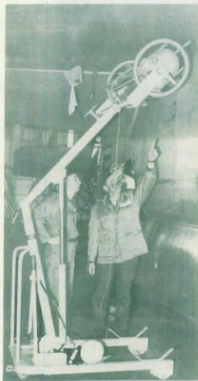
X ray machine being positioned to photograph B-66 wing doubler. This will permit locating cracks without removing wing skin.
